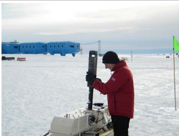
Jonathan Shanklin with a Dobson ozone spectrophotometer at Halley Research Station
